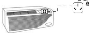
The grounding wire of the packaged terminal air conditioner must be firmly connected to the grounding wire of the power source. Improper grounding will lead to possible electric shock or other hazards.
