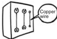
Improper use of metal wires, copper wires for the fuse may result in faulty performances of the machine or fire hazards.
